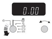
To set the clock to read the time of day turn and hold the Setting knob to the clock symbol ( ) and at the same time turn the Adjusting knob left or right until the clock shows the time of day. This is a 12 hour clock. Let go of the Setting knob and it will spring back to the vertical ( ) oven manual setting.
